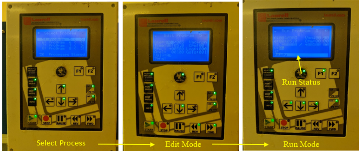
Figure 4: Control Panel Process
